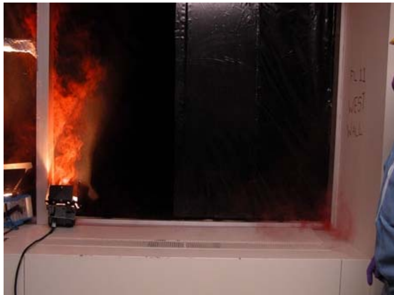
Figure 6. Smoke test of window mullions.
